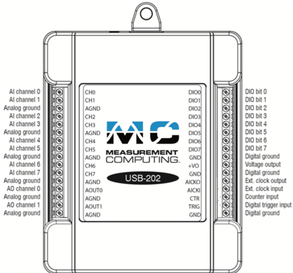
Figure 3. USB-202 pinout
