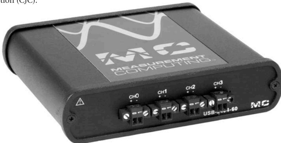
The USB-2404-10 and USB-2404-60 (shown above) each provide four 24-bit simultaneous-sampling analog inputs with sample rates up to 50 kS/s per channel and up to 250 Vrms channel-to-channel and channel-to-ground isolation. The USB-2404-10 supports an input voltage range of  $\pm 10$  V, and the USB-2404-60 supports a range of  $\pm 60$  V.
