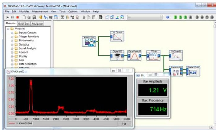
*DASYLab gives users the ability to create applications by simply dragging-and-dropping functional icons on a worksheet, connecting the icons together, and running the program. DASYLab supports most MCC data acquisition hardware.*
