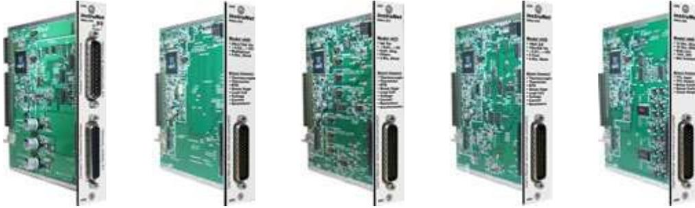
instruNet i4xx cards are installed by the end user into an instruNet card cage that is 4, 8, 12 or 16 slots wide. Each card is 13 x 2.5 x 13 cm in size. Below is a list of available cards.
