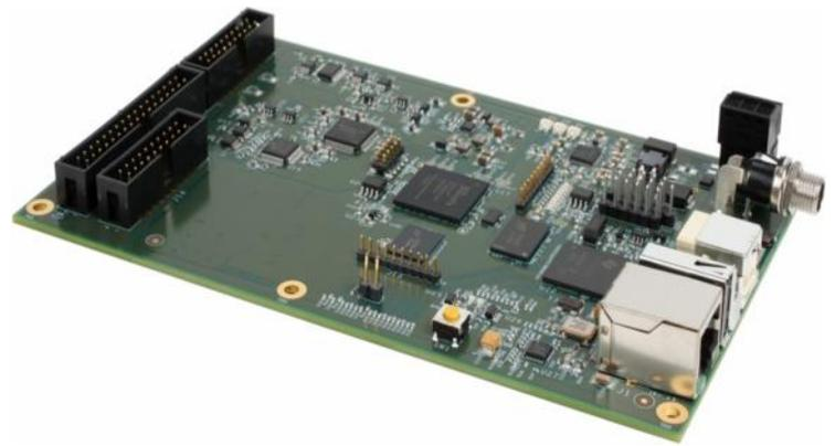
**Figure 1. The DT7816 provides 8 analog inputs, 2 analog outputs, DIO, C/T, tachometer, and measure counter functions along with an embedded ARM processor for real-time processing and analysis of DAQ measurements.**
