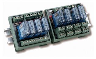
**Introduction:** RM series relay modules are designed to be mounted on DIN RAIL TS-15,TS-32 or TS-35. RM-10X contains SPDT relays, while RM-20X contains DPDT relays. In order to prevent improper operation, reverse polarity protection is provided. The status of each channel is indicated by an LED. These relay modules are provided in 4,8 or 16 channel versions.
