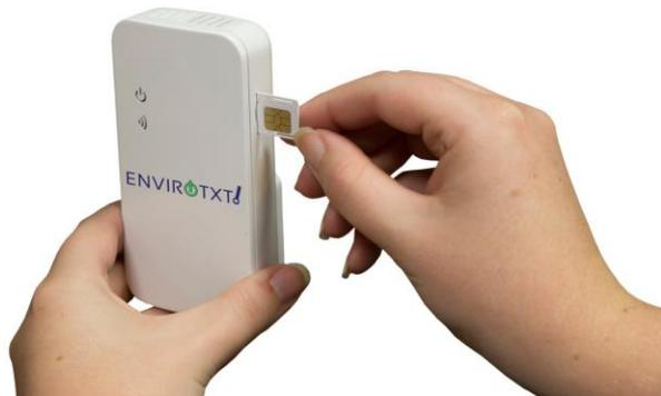
*Inserting a SIM Card*
