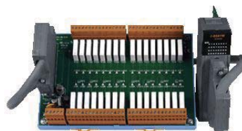
I-87041W, I-87041PW with DN-8K32R and DB37 Male to Female Cable (Optional)
